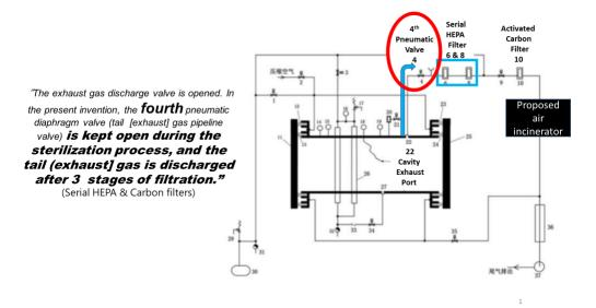
Figure 62. Graphic depiction of Biosafety Autoclave contained in the April 22, 2019 WIV patent describing changes to the design and procedures. The insertion of the proposed November 19, 2019 procurement of an air incinerator is superimposed on the graphic as it was described in the procurement notice. Source: *Wuhan Institute of Virology. 2019. Patent: No. 201910325059.0 Biosafety autoclave and sterilization method.*
