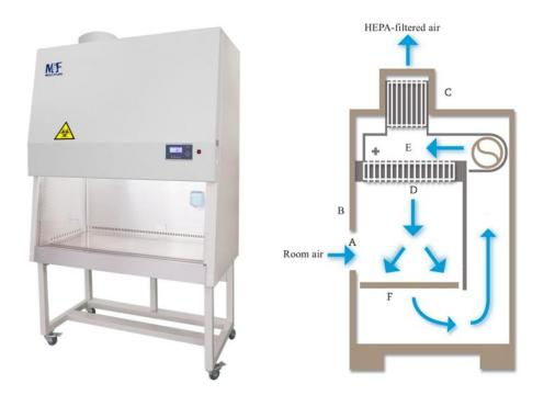
Figure 47. Graphic depiction Biosafety Cabinet and negative airflow with high-efficiency particulate (HEPA) filter Source: Biosafety Cabinets. <u>https://ehs.umass.edu/sites/default/files/Biosafety%20Cabinets.pdf</u>
